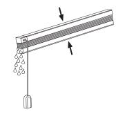
Position the wet pleated blind on the holding clip and clip it into the holding clip by slightly tilting the rail.
